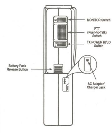
Battery Pack Release Button - To remove the Battery Pack, push up on the release button and slide the Battery Pack away from the radio.
